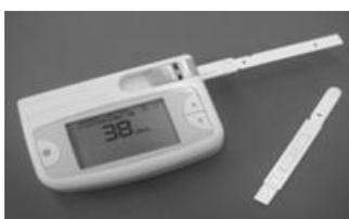
**Figure 13:** Portable sAA biosensor comprising a handheld reader and a disposable collection strip [78].
