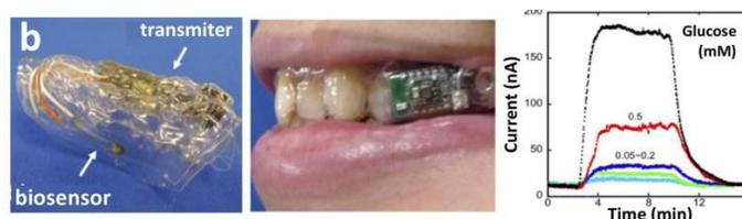
**Figure 11:** Saliva glucose sensor "mouth guard" [52].
