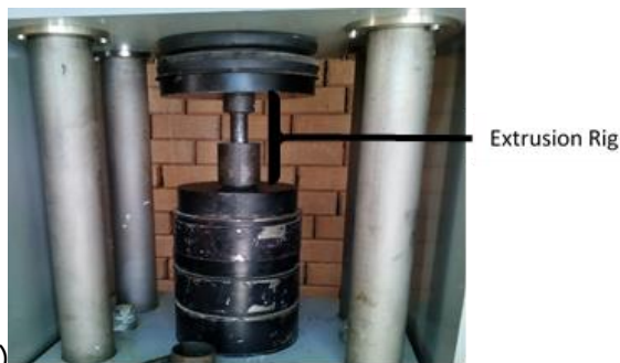
Figure 4: (a)- Plate 9: Machine Aluminium 6063-Alloy Billet; (b)- Plate 10: 2000KN Capacity UT CO821 Compress Machine and Extrusion Rig Setup
