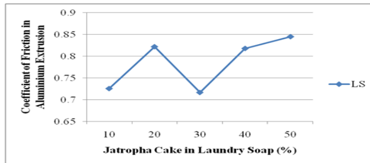
Figure 7: Variation of Coefficient of Friction in Aluminium Extrusion with Percentage Jatropha Cake in Savon (Laundry Soap).
