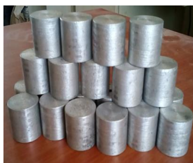
Figure 4: (a)- Plate 9: Machine Aluminium 6063-Alloy Billet; (b)- Plate 10: 2000KN Capacity UT CO821 Compress Machine and Extrusion Rig Setup
