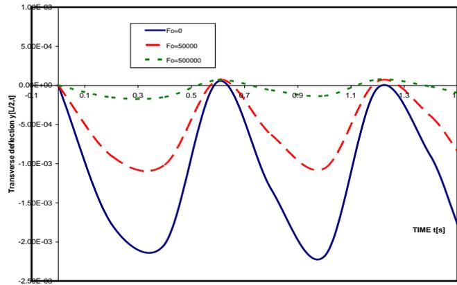
**Figure3:** Deflection profile of a simply supported structurally damped thin beam resting on exponentially decaying foundation and subjected to Harmonic variable magnitude moving loads for various values of foundation modulus  $F_0$ .
