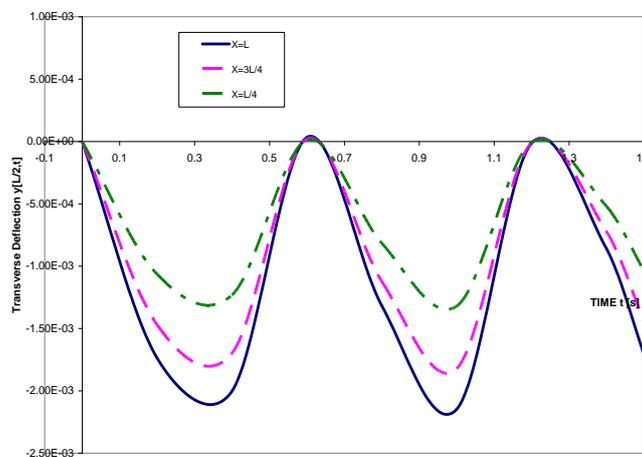
**Figure 4:** Transverse displacement response of a simply supported structurally damped thin beam resting on exponentially decaying foundation and subjected to Harmonic variable magnitude moving loads for various values of spatial coordinates and for fixed value of foundation modulus  $F_0 = 4000$ .
