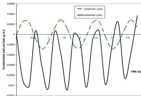
**Figure 5:** Comparison of the response of the simply supported structurally damped thin beam to constant and variable magnitude moving distributed load for foundation modulus  $F_0 = 4000$ .
