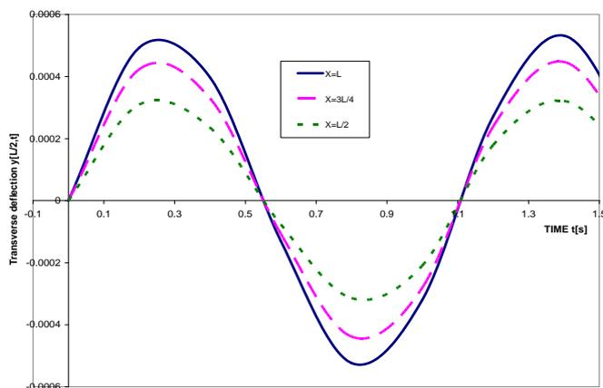
**Figure 2:** Transverse displacement response of a simply supported structurally damped thin beam resting on exponentially decaying foundation and subjected to constant magnitude moving loads for various values of spatial coordinates x and for fixed value of foundation modulus  $F_0 = 4000$ .
