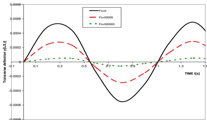
**Figure 1:** Displacement response of a simply supported structurally damped thin beam resting on exponentially decaying foundation and subjected to constant magnitude moving loads for various values of foundation modulus  $F_0$ .
